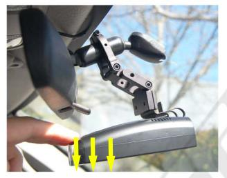
9 - To access the buttons of the RD you will need to gently push downward on the front of the RD with one finger and push the desired button with another finger. Then allow the RD to return to it's original position by gently letting it spring upward. When accessing the buttons, be sure to push the RD downward just enough for your finger to fit between the RD and mirror. Do not push down more than what is needed.
